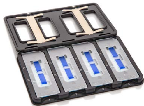
Figure 1: The Cell Chip adapter – four chips (eight samples) can be loaded and analyzed in one measurement run.
